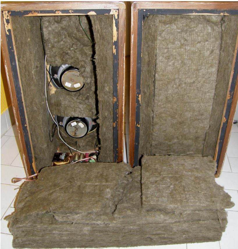
Putting back the many layers of glass wool.
